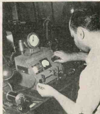
The insulating value of the enamel coating on fine wire produced at the Dobbs Ferry plant of North American Phillips is checked on this instrument
