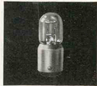
NE-17 Indicator and pilot light lamp that flashes to show condition of B-battery in portable radios. Frequency of flashes decreases as battery runs down.
