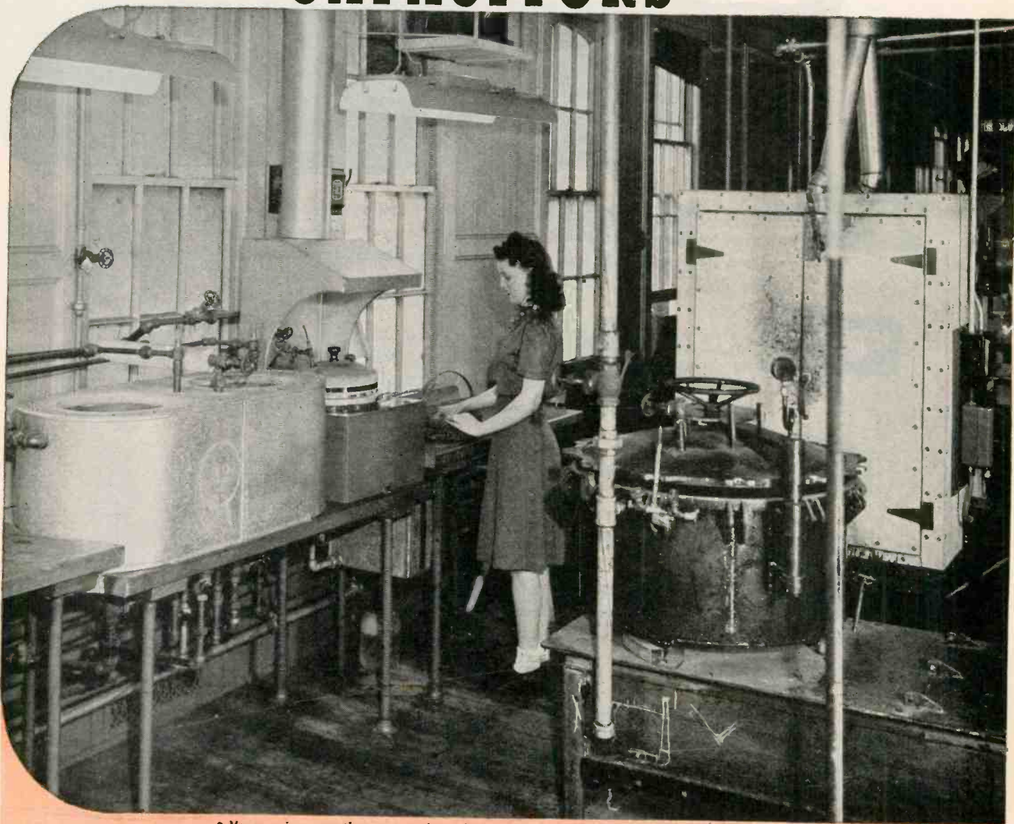
• Vacuum impregnation tank and waxing equipment for special treatment of mica films.
