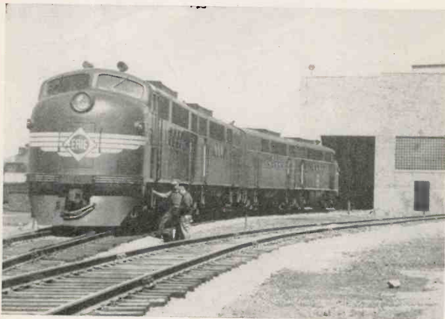
When diesel locomotives approach this Erie maintenance shop, the headlamp shines into a phototube which actuates a door opener and eliminates a preliminary stop while trainmen open the door
