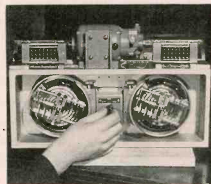
This switch is being set for eight-channel service and also permits selection of two or four channels. At each side of the switch is a face-plate mechanism that feeds to or from the seven-unit printing equipment
