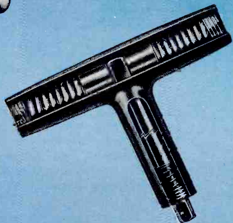
THE NOW FAMOUS SKYWAY "T" torque wrench — tested and used by the Army Air Forces. An absolute torque limiting action incorporating a ratcheting shaft for production speed use. Range in two models, 0-25 inch pounds and 25-90 inch pounds.
