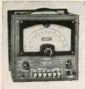
Condenser Tester Model 650A—Measures Capacity, Power Factor and Leakage
